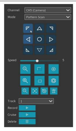
Pattern Scan: Pattern scanning refers to the scanning according to the pre-set path, recording the horizontal and vertical movement, multiplier operation and other actions of the PTZ. After recording and saving, the pattern scanning route can be directly called. This function supports setting 4 pattern scan paths and provides saving options for each pattern scan path.
